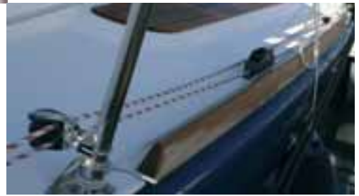
Continuous furling line installed with a jammer
